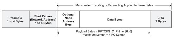
The Preamble, Start Pattern and CRC bytes are added to the packet by the TRC103 during transmit and removed from the packet during receive.
