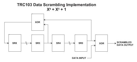
All 9 shift registers preset to 1 before each scrambling (DC balancing) calculation
