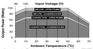
**Derating requirements** – Chart above applies to models 1003 thru 1008 only. 100W 300 LFM forced air, open frame. 70W convection cooled open frame. Derate 10% with Chassis and Cover. Derate 1.0Wout / 1VIN below 100VIN and between 100VIN and 85VIN. Use larger of the two deratings when using chassis/cover below 100VIN. Derate output power linearly to 50% between 50° and 70°C.
