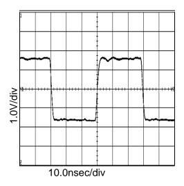
Figure 10. 16.9MHz Output Waveform (V<sub>DD</sub>=3.3V, at C<sub>L</sub>=15pF)
