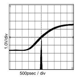
Figure 17. 18.4MHz Period-Jitter (V<sub>DD</sub>=3.3V, at C<sub>L</sub>=15pF)
