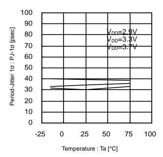
Figure 35. Period-Jitter 1σ vs Temperature (18.4MHz)
