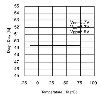
Figure 22. Duty vs Temperature (27MHz)
