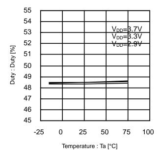
Figure 19. Duty vs Temperature (54MHz)
