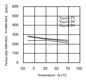
Figure 27. Period-Jitter MIN-MAX vs Temperature (33.9MHz)
