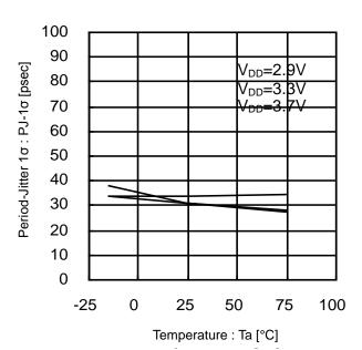
Figure 32. Period-Jitter 1 $\sigma$  vs Temperature (36.9MHz)
