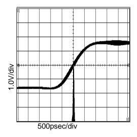
Figure 14. 36.9MHz Period-Jitter (V<sub>DD</sub>=3.3V, at C<sub>L</sub>=15pF)
