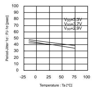
Figure 26. Period-Jitter 1σ vs Temperature (33.9MHz)
