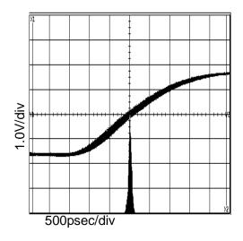
Figure 2. 54MHz Period-Jitter (V<sub>DD</sub>=3.3V, at C<sub>L</sub>=15pF)
