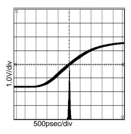
Figure 8. 33.9MHz Period-Jitter  $(V_{DD}=3.3V, at C_L=15pF)$
