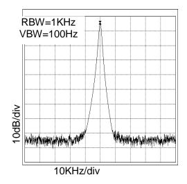
Figure 6. 27MHz Spectrum (V<sub>DD</sub>=3.3V, at C<sub>L</sub>=15pF)
