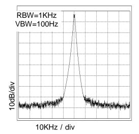
Figure 18. 18.4MHz Spectrum ( $V_{DD}$ =3.3V, at  $C_L$ =15pF)
