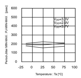
Figure 36. Period-Jitter MIN-MAX vs Temperature (18.4MHz)
