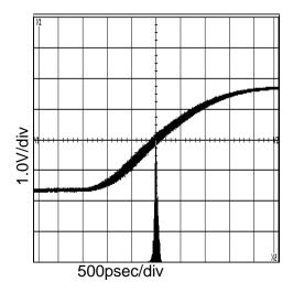
Figure 5. 27MHz Period-Jitter (V<sub>DD</sub>=3.3V, at C<sub>L</sub>=15pF)
