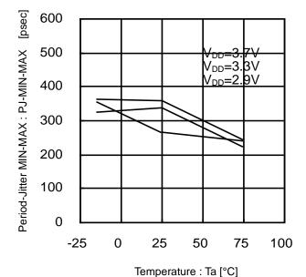
Figure 30. Period-Jitter MIN-MAX vs Temperature (16.9MHz)
