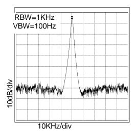
Figure 12. 16.9MHz Spectrum (V<sub>DD</sub>=3.3V, at C<sub>L</sub>=15pF)
