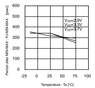
Figure 21. Period-Jitter MIN-MAX vs Temperature (54MHz)
