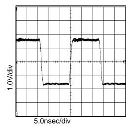
Figure 13. 36.9MHz Output Waveform (V<sub>DD</sub>=3.3V, at C<sub>L</sub>=15pF)
