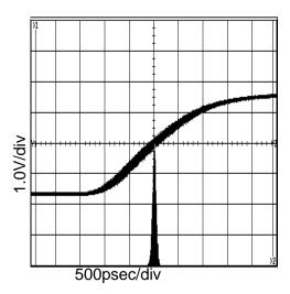
Figure 11. 16.9MHz Period-Jitter (V<sub>DD</sub>=3.3V, at C<sub>L</sub>=15pF)
