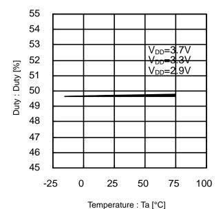
Figure 25. Duty vs Temperature (33.9MHz)
