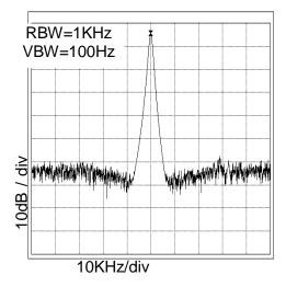
Figure 9. 33.9MHz Spectrum (V<sub>DD</sub>=3.3V, at C<sub>L</sub>=15pF)
