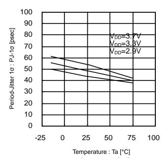
Figure 29. Period-Jitter 1σ vs Temperature (16.9MHz)
