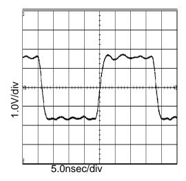
Figure 4. 27MHz Output Waveform ( $V_{DD}$ =3.3V, at  $C_L$ =15pF)
