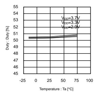
Figure 31. Duty vs Temperature (36.9MHz)
