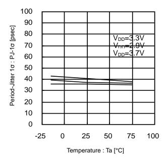
Figure 23. Period-Jitter 1σ vs Temperature (27MHz)
