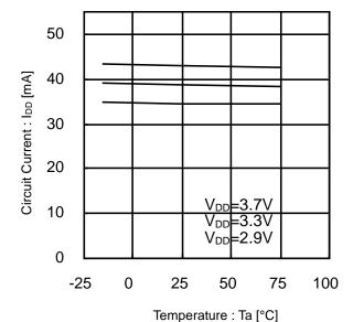
Figure 37. Consumption Current vs Temperature
