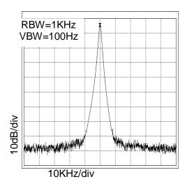
Figure 15. 36.9MHz Spectrum  $(V_{DD}=3.3V, at C_L=15pF)$
