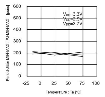
Figure 33. Period-Jitter MIN-MAX vs Temperature (36.9MHz)
