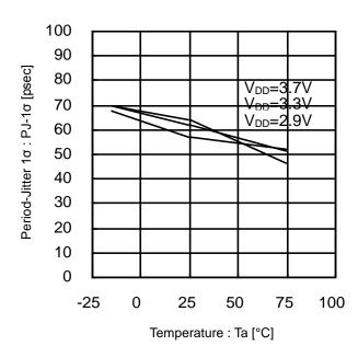
Figure 20. Period-Jitter 1 $\sigma$  vs Temperature (54MHz)
