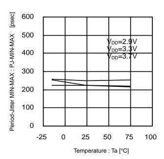
Figure 24. Period-Jitter MIN-MAX vs Temperature (27MHz)
