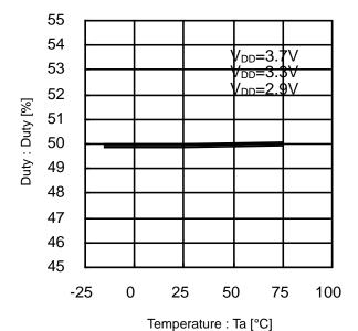
Figure 34. Duty vs Temperature (18.4MHz)
