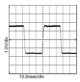
Figure 16. 18.4MHz Output Waveform  $(V_{DD}=3.3V, at C_{L}=15pF)$
