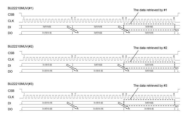
Figure 14. Communication Format of three BU22210MUVs cascade connection
