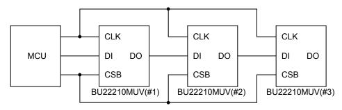
Figure 13. Example configuration of three BU22210MUVs cascade connection
