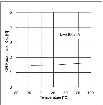
Figure 6. ON-Resistance vs Temperature (Voltage Driver Block)
