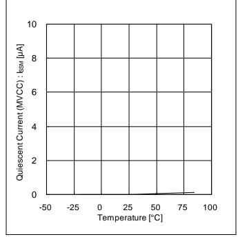
Figure 4. Quiescent Current (MVCC) vs Temperature
