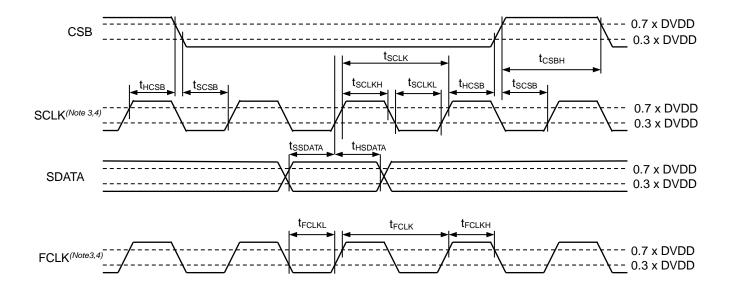
(Note 3) FCLK is asynchronous with SCLK. (Note 4) The duty of FCLK and SCLK is arbitrary after observing the above table.
