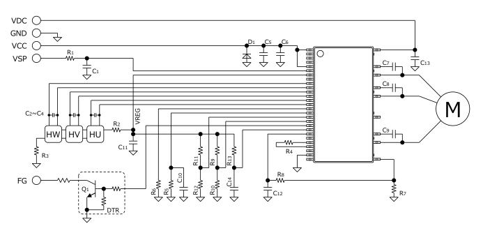
Figure 48. Application Example (180° Sinusoidal Commutation Driver, CCW="H", FGS="H")
