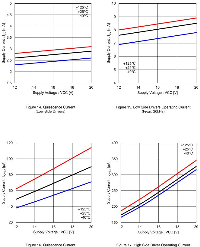
Figure 17. High Side Driver Operating Curre (f<sub>PWM</sub>: 20kHz, Each Phase)
