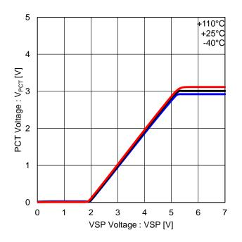
Figure 32. VSP vs PCT Offset Voltage
