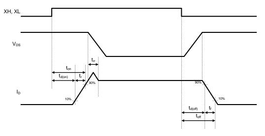
Figure 12. Switching Time Definition
