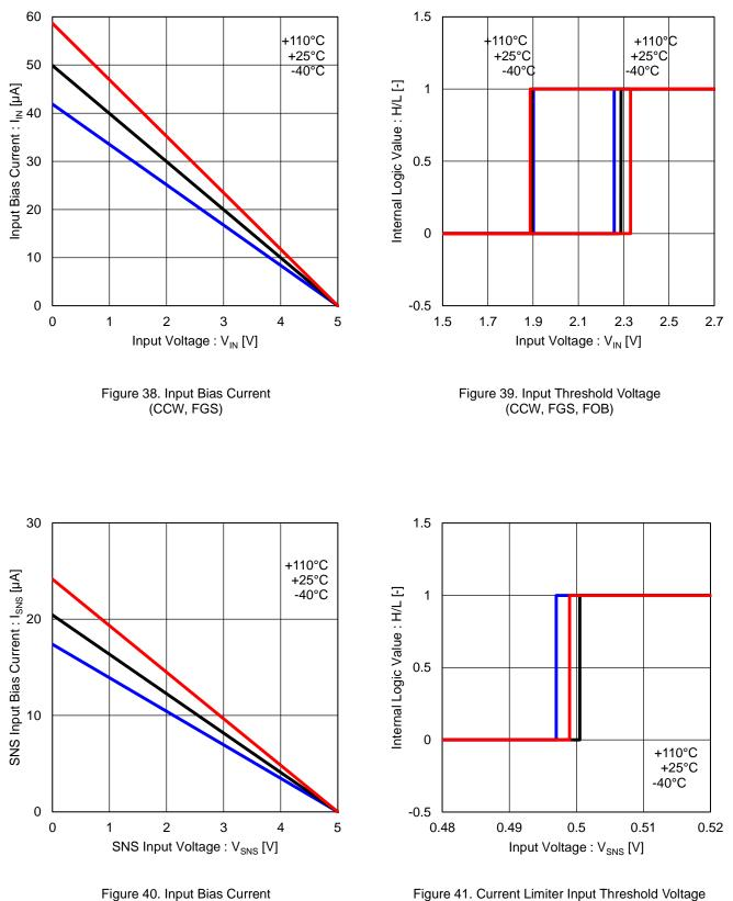
Figure 41. Current Limiter Input Threshold Voltage (SNS)
