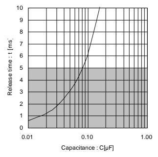
Figure 9. Release Time (Reference Data @R=100k $\Omega$ )
