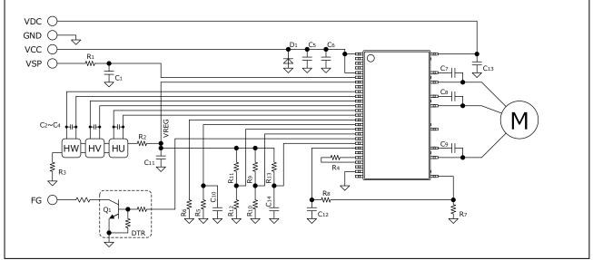
Figure 1. Application Circuit Example
