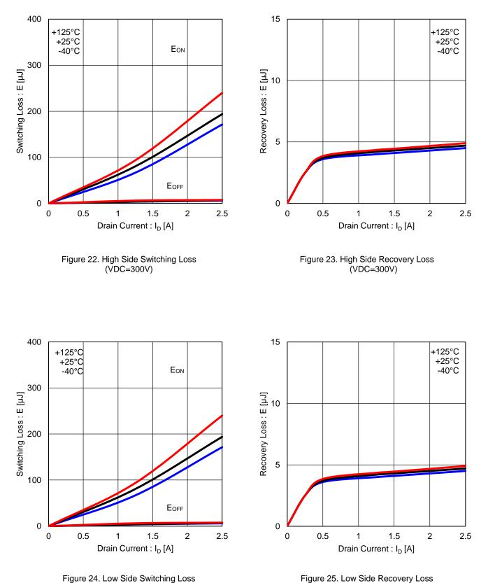
Figure 25. Low Side Recovery Loss (VDC=300V)
