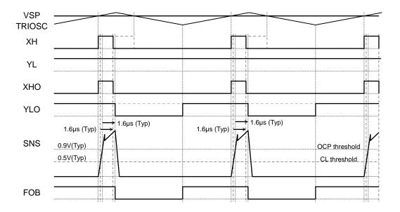
Figure 7. Fault Operation ~ OCP ~ Timing Chart
