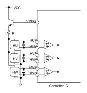
Figure 6. VREG Output Pin Application Example
