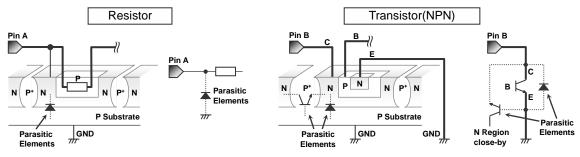
Figure 60. Example of IC structure
