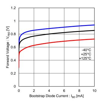
Figure 20. Bootstrap Diode Forward Voltage
