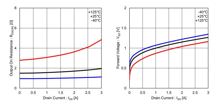
Figure 18. Output MOSFET ON Resistance
