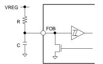
Figure 8. Release Time Setting Application Circuit
