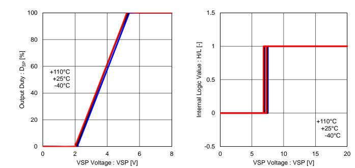
Figure 30. Output Duty vs VSP Voltage
