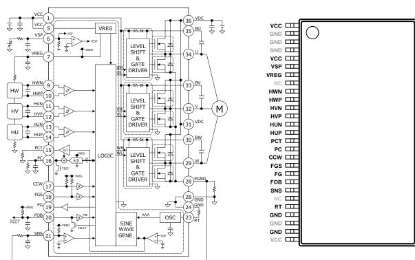
Figure 2. Block Diagram
