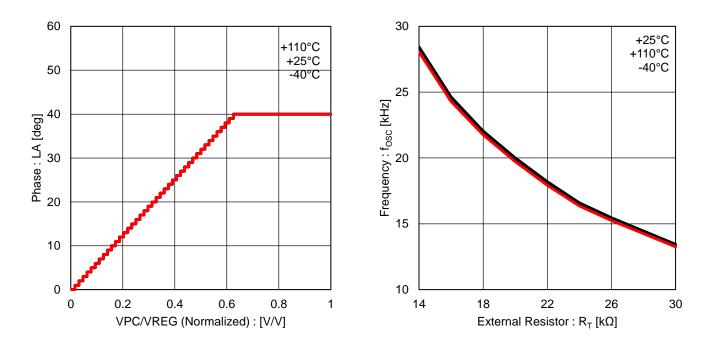
Figure 34. PC Voltage Normalized vs Lead Angle
