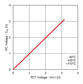
Figure 33. PCT vs PC Linearity ( $R_{PCT}=R_{PC}=100k\Omega$ )
