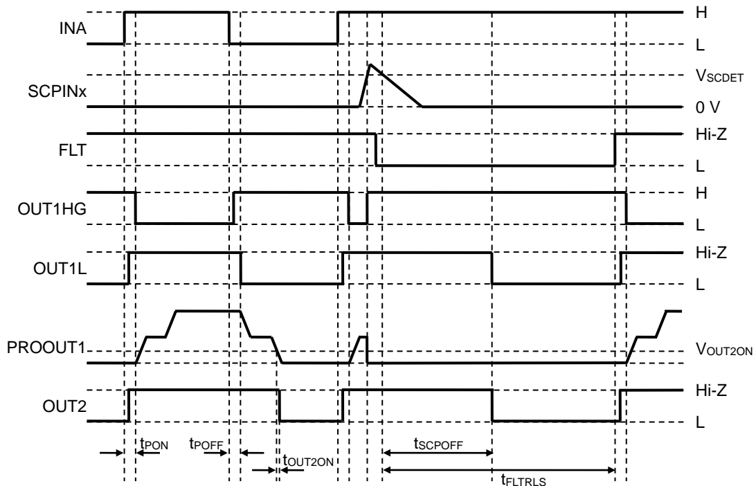
Figure 81. Timing Chart of Miller Clamp Function
