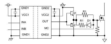
Figure 32. Driving Si MOSFET with Buffer Circuit
