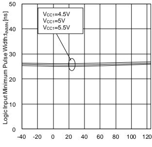
Figure 18. Logic Input Minimum Pulse Width vs Temperature
