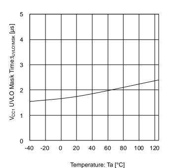
Figure 28. V<sub>CC1</sub> UVLO Mask Time vs Temperature
