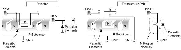
Figure 33. Example of IC structure
