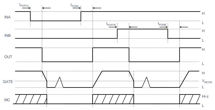
Figure 3. Timing Chart of Miller Clamp Function
