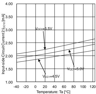
Figure 10. Input-side Circuit Current 2 vs Temperature (At INA=100 kHz, Duty=50 %)
