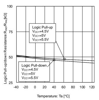
Figure 17. Logic Pull-up/down Resistance vs Temperature
