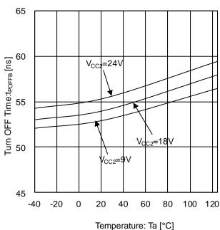
Figure 24. Turn OFF Time vs Temperature (INA=H, INB=PWM)
