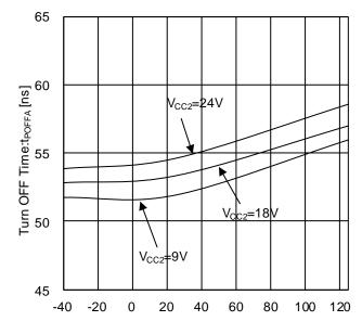
Figure 22. Turn OFF Time vs Temperature (INA=PWM, INB=L)
