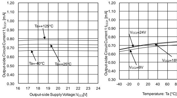
Figure 11. Output-side Circuit Current 1 vs Output-side Supply Voltage (At OUT=L)
