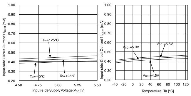
Figure 7. Input-side Circuit Current 1 vs Input-side Supply Voltage
