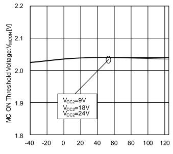
Figure 26. MC ON Threshold Voltage vs Temperature
