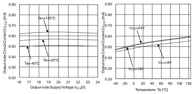
Figure 13. Output-side Circuit Current 2 vs Output-side Supply Voltage (At OUT=H)
