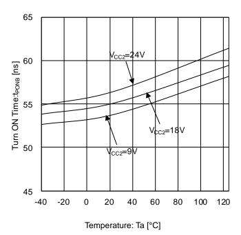
Figure 23. Turn ON Time vs Temperature (INA=H, INB=PWM)
