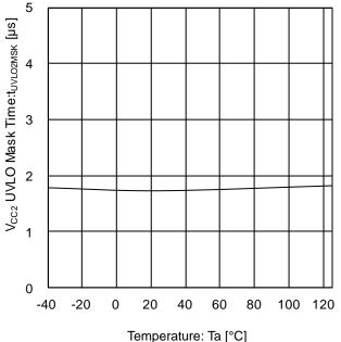
Figure 30. V<sub>CC2</sub> UVLO Mask Time vs Temperature
