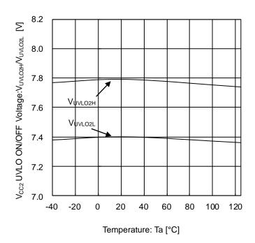
Figure 29. V<sub>CC2</sub> UVLO ON/OFF Voltage vs Temperature
