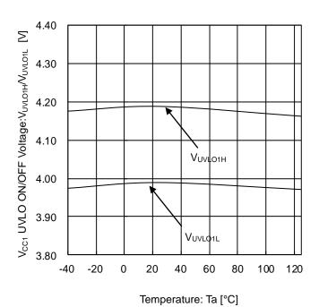
Figure 27. V<sub>CC1</sub> UVLO ON/OFF Voltage vs Temperature
