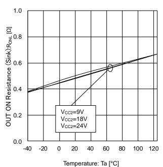
Figure 20. OUT ON Resistance (Sink) vs Temperature
