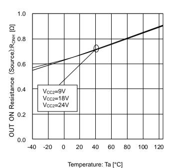
Figure 19. OUT ON Resistance (Source) vs Temperature
