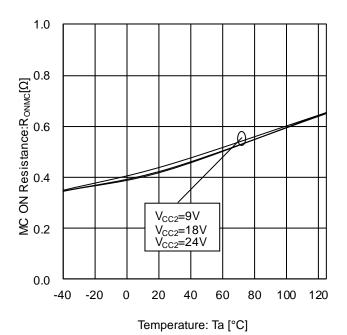
Figure 25. MC ON Resistance vs Temperature
