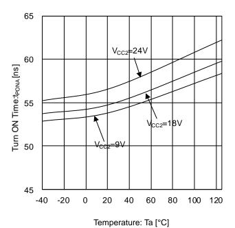
Figure 21. Turn ON Time vs Temperature (INA=PWM, INB=L)
