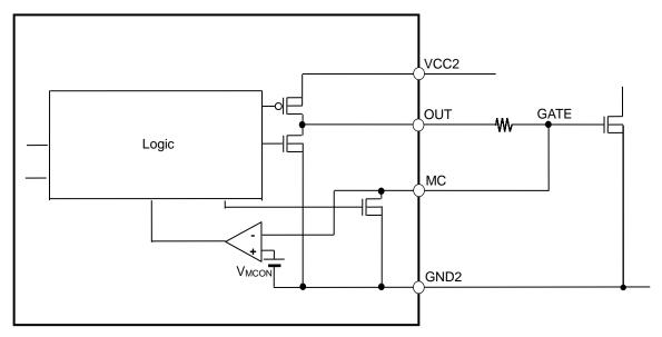
Figure 2. Block Diagram of Miller Clamp Function
