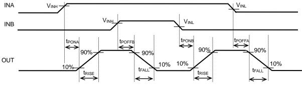
Figure 6. Timing Chart of IN-OUT
