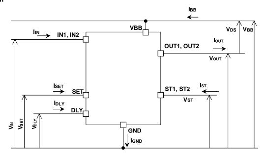
Figure 1. Voltage and Current Definition
