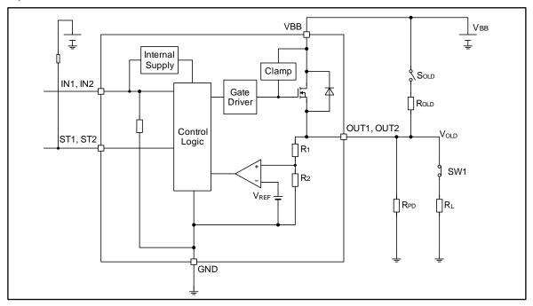
Figure 38. Open Load Detection Block Diagram
