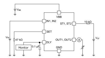
Figure 30. Fixed Over Current Limit Variable Over Current Limit
