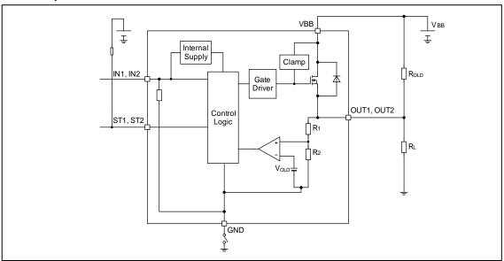
Figure 40. GND Open Protection Block Diagram
