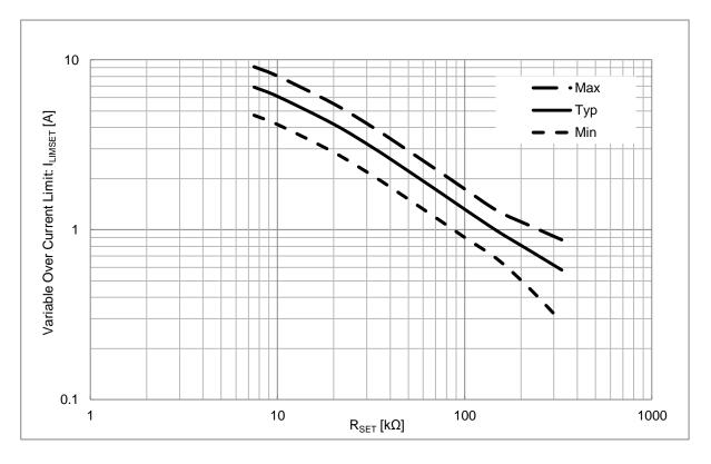
Figure 36. Variable Over Current Limit vs  $R_{\text{SET}}$
