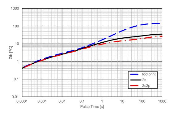
Figure 5. Transient Thermal Resistance
