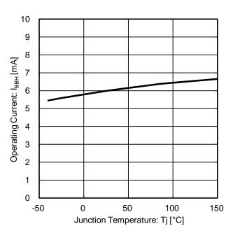
Figure 9. Operating Current vs Junction Temperature
