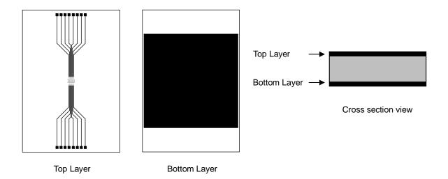
Figure 3. PCB Layout (2s)
