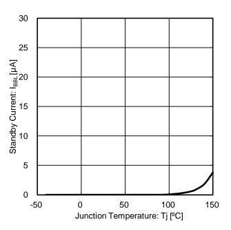
Figure 7. Standby Current vs Junction Temperature
