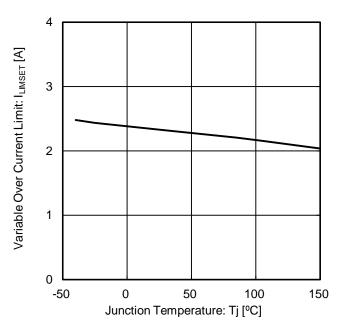
Figure 21. Variable Over Current Limit vs Junction Temperature
