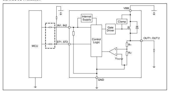
Figure 41. MCU I/O Protection
