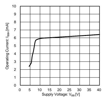
Figure 8. Operating Current vs Supply Voltage
