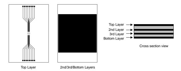
Figure 4. PCB Layout (2s2p)
