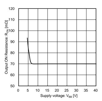
Figure 13. Output ON Resistance vs Supply Voltage
