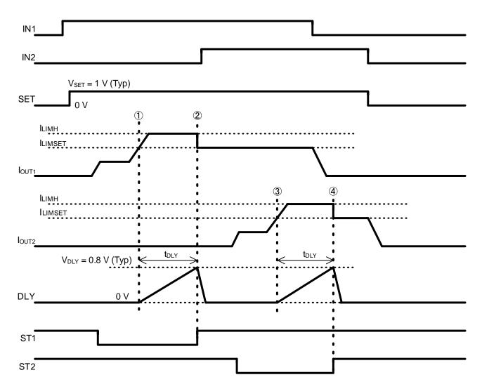
Figure 34. Timing Chart for Over Current Detection in Both Outputs
