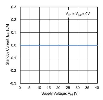
Figure 6. Standby Current vs Supply Voltage
