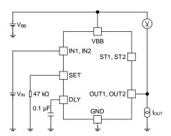
Figure 27. Output ON Resistance Output Clamp Voltage
