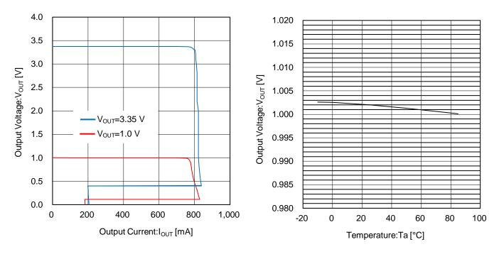
Figure 17. Output Voltage vs Output Current
