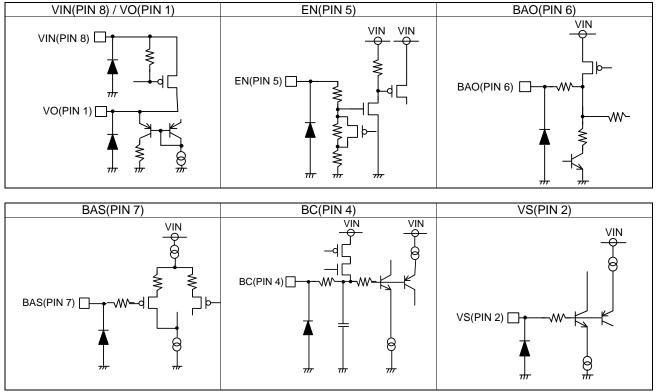
Figure 38. I/O Equivalence Circuits
