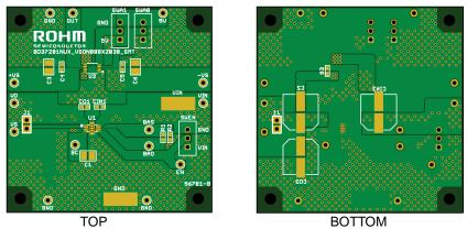
(board size 60mm x 60mm, board thickness 1.6mm, material FR-4)
