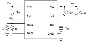
Figure 36. External Components Connection
