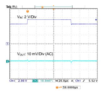
Figure 29. Line Transient (I<sub>OUT</sub>=500 mA Slew Rate=1 V/µs V<sub>OUT</sub>=3.35 V)
