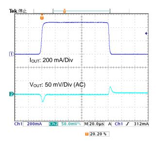
Figure 32. Load Transient (I\_{OUT}=0 mA to 500 mA V\_{OUT}=1.0 V)
