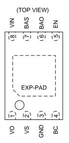
Figure 2. Pin Configuration
