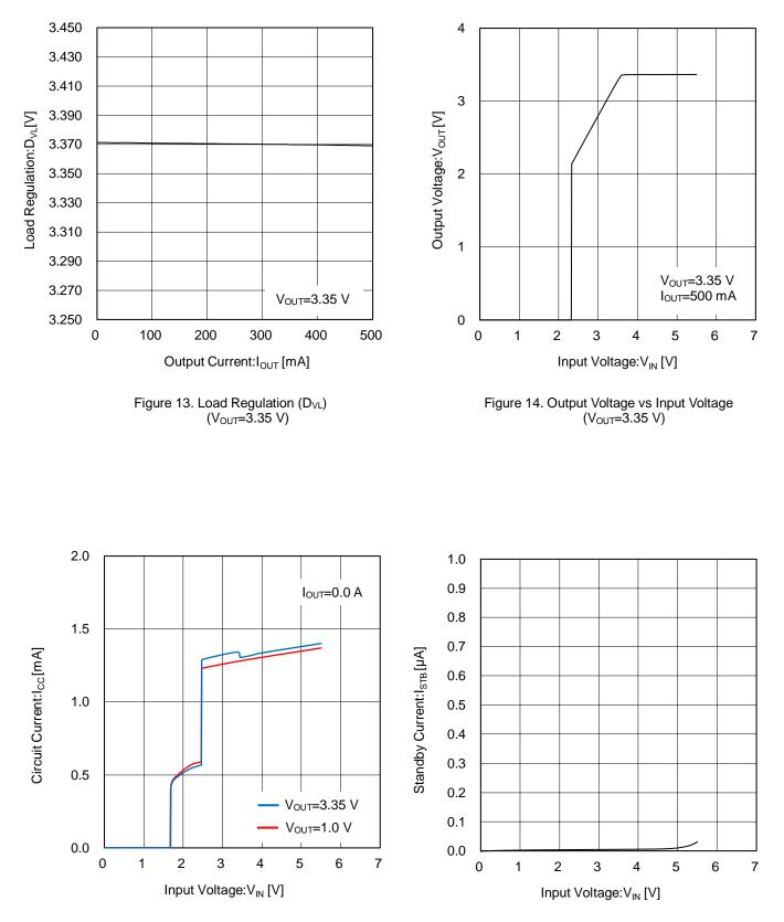
Figure 15. Circuit Current vs Input Voltage
