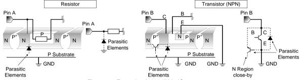
Figure 40. Example of monolithic IC structure
