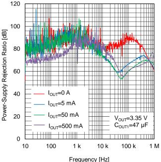
Figure 22. Power-Supply Rejection Ratio (V<sub>OUT</sub>=3.35 V)
