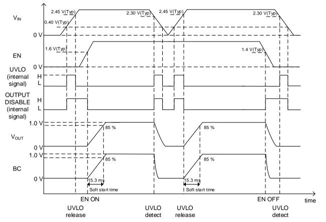
Figure 4. The Sequence Waveform During V<sub>IN</sub>/EN Rising and Falling (When at BC Capacitor 1  $\mu$ F and V<sub>OUT</sub> 1.0 V Settings)
