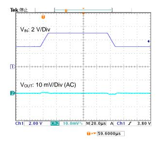
Figure 30. Line Transient (I\_OUT=500 mA Slew Rate=0.2 V/µs V\_OUT=1.0 V)
