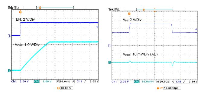
Figure 27. Soft Start (V<sub>OUT</sub>=3.35 V)
