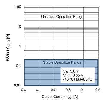
Figure 37. ESR of COUT1 vs Output Current
