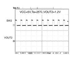
Fig.19 SW2 wave form (Io=1.5A)
