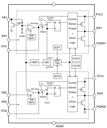
Fig.2 BD9152MUV Block Diagram
