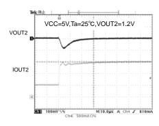
Fig.22 VOUT2 transient responce (Io0.5A→1.5A/ usec)
