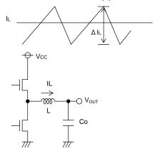
Fig.33 Output ripple current
