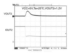
Fig.23 VOUT2 transient responce (Io1.5A→0.5A/ usec)
