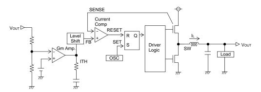
Fig.27 Diagram of current mode PWM control
