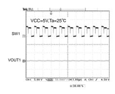
Fig.16 SW1 wave form (Io=0mA)
