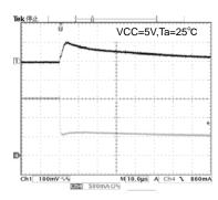
Fig.21 VOUT1 transient responce (Io1.5A→0.5A/ usec)
