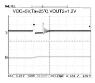
Fig.18 SW2 wave form (Io=0mA)
