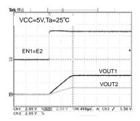
Fig.15 Soft start wave form (Io=1.5A)
