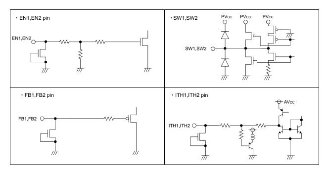
Fig.41 I/O equivalence circuit
