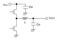
Fig.35 Input capacitor
