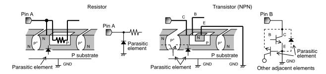
Fig.42 Simplified structure of monorisic IC
