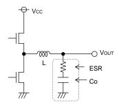
Fig.34 Output capacitor
