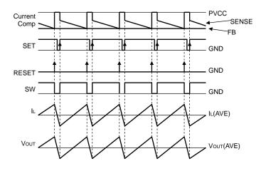
Fig.28 PWM switching timing chart
