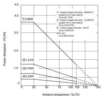
Fig.32 Thermal derating curve (VQFN020V4040)
