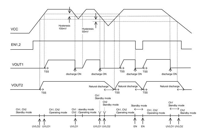
Fig.30 Soft start, Shutdown, UVLO timing chart
