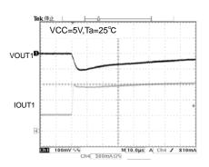
Fig.20 VOUT1 transient responce (Io0.5A→1.5A / usec)
