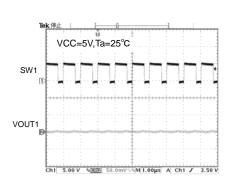
Fig.17 SW1 wave form (Io=1.5A)
