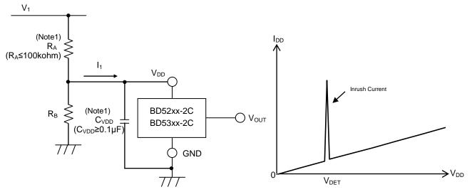
Figure 36. Resistor Divider Connection Application
