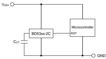
Figure 34. CMOS Output type
