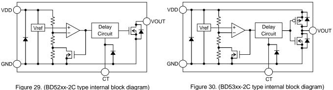
Figure 29. (BD52xx-2C type internal block diagram)
