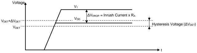
Figure 40. V<sub>DD</sub> Drop Caused by Inrush Current
