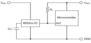
Figure 1. Open Drain Output Type BD52xx-2C Series
