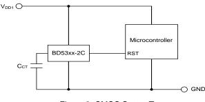
Figure 2. CMOS Output Type BD53xx-2C Series
