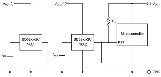
Figure 35. OR Circuit Connection Application
