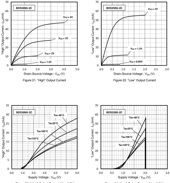
Figure 23. "High" Output Current (V<sub>DS</sub>=0.5V)
