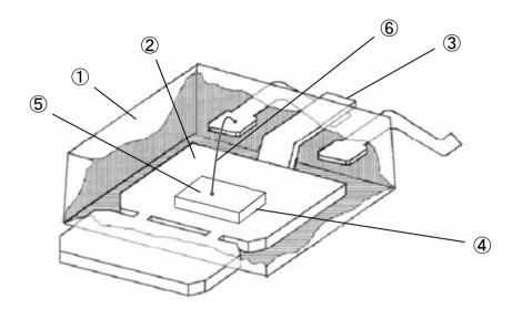
\* A direction of wire bonding and die bonding, a pattern of die bonding, and a shape of frame differ by a form name.
