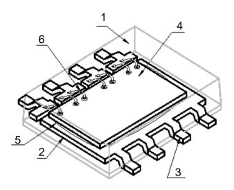
A direction of wire bonding and die bonding, a shape of frame, die size and the number of wires differ by P/N.
