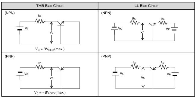
Built-in resistor of digital transistors omitted
