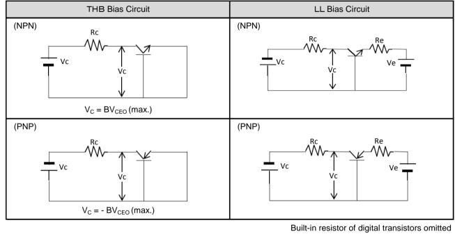
\*3 Method of test 1, test 2
