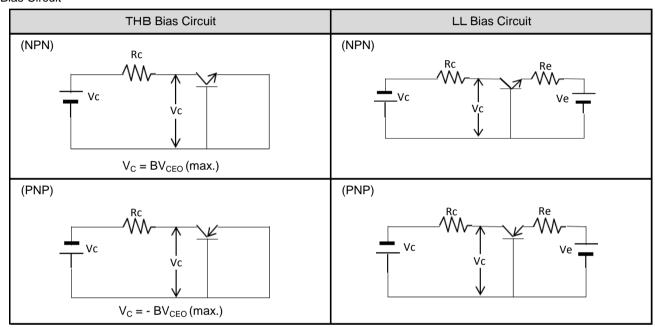
Built-in resistor of digital transistors omitted
