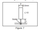
Soldering directly to the case will reduce the degree of vacuum and may result in deterioration of the characteristics and may break the crystal chip.
