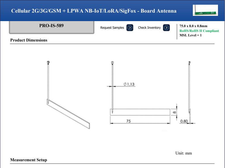
The antenna measurements were done on a standard measurement fixture - the antenna mounted in an ABS plastic box, 150x150x45 mm, connected to a PCB, 120x50 mm, with the cable fully extended
