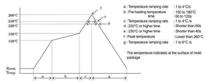
(1) Using reflow furnace with short wave infrared radiation heater such halogen lamp regarding temperature profile. Please refer to those of reflow furnace.
