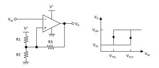
Figure 7. Inverting Comparator with Hysteresis
