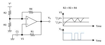
Figure 11. Square Wave Oscillator
