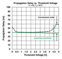
Figure 3. Propagation delay vs. Threshold Voltage
