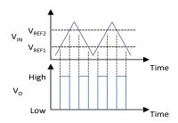
Figure 10. Window comparator output results
