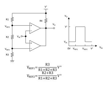
Figure 9. Window Comparator with NJU7726x
