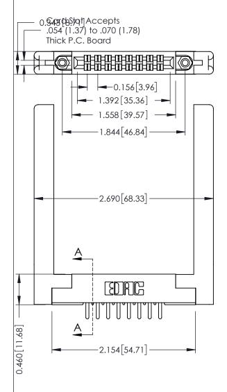
SECTION A-A 0.295[7.49] Card Slot 0.090 [2.29] Point of Contact 305 ENG MASTER 305 / 315 / 355 Card Edge Connector
