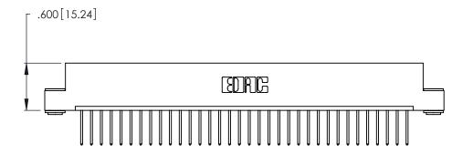
Card Slot Accepts .054 [1.37] to .070 [1.78] Thick P.C. Board .330 [8.38] Card Slot .160 [4.07] Point of Contact
