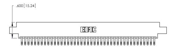
Card Slot Accepts .054 [1.37] to .070 [1.78] Thick P.C. Board .330 [8.38] Card Slot .160 [4.07] Point of Contact
