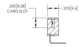
**Contact Dimensions:** 558-90 Degree Bend (Code 541 Contacts) See Sheet 2 for Contact Code 555, 556, 558, 559, 560 Dimensions
