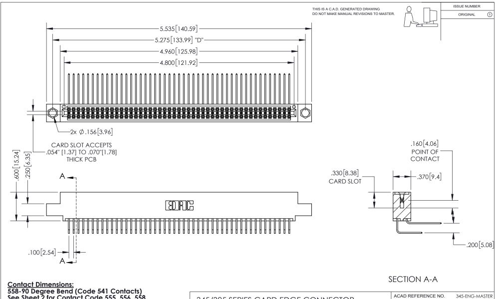
558-90 Degree Bend (Code 541 Contacts) See Sheet 2 for Contact Code 555, 556, 558, 559, 560 Dimensions
