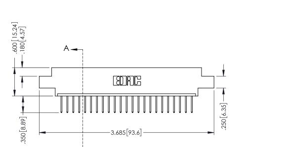
.330 [8.38] Slot Depth .160 [4.06] Point of Contact **SECTION A-A**
