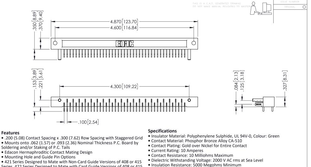
Series, 422 Series Designed to Mate with Card Guide Versions of 408 or 415 Series, 423 Series Designed to Mate with 424 or 438 Series
