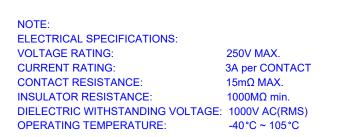
MATERIAL & FINISH: HOUSING: PBT, UL94V-0 CONTACTS: PHOSPHOR BRONZE, TIN PLATED SEALS: SILICONE RUBBER
