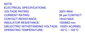
MATERIAL & FINISH: HOUSING: PBT, UL94V-0 CONTACTS: PHOSPHOR BRONZE, TIN PLATED SEALS: SILICONE RUBBER
