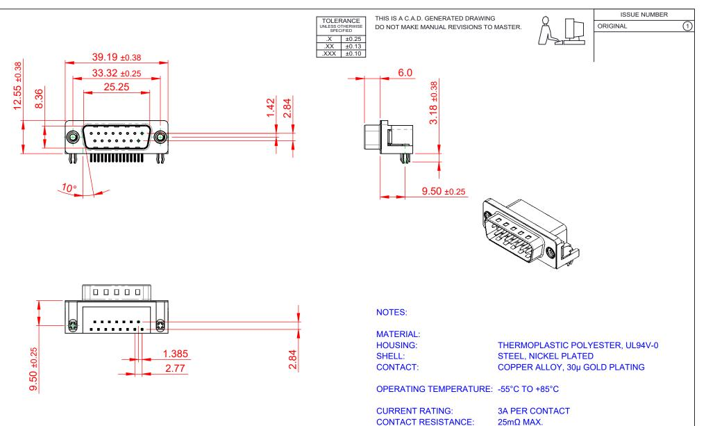
**INSULATOR RESISTANCE:** DIELECTRIC WITHSTANDING VOLTAGE: 1000V AC rms
