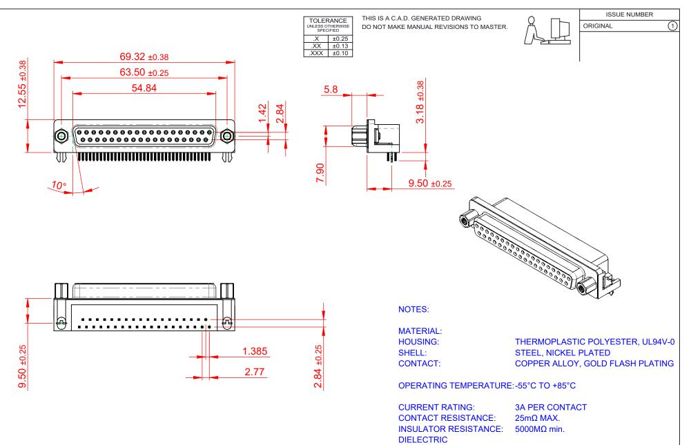
WITHSTANDING VOLTAGE: 1000V AC rms
