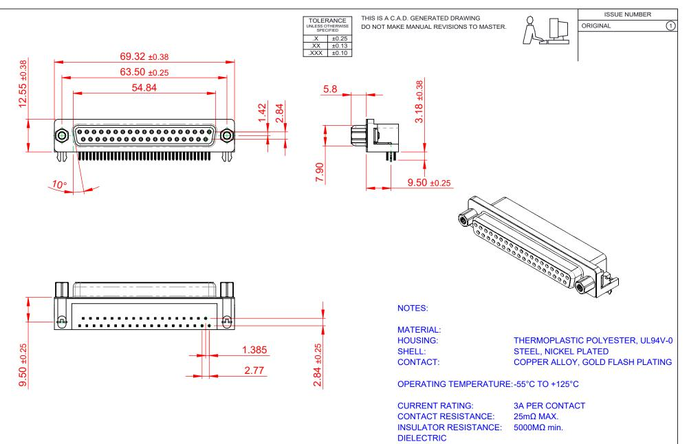
WITHSTANDING VOLTAGE: 1000V AC rms
