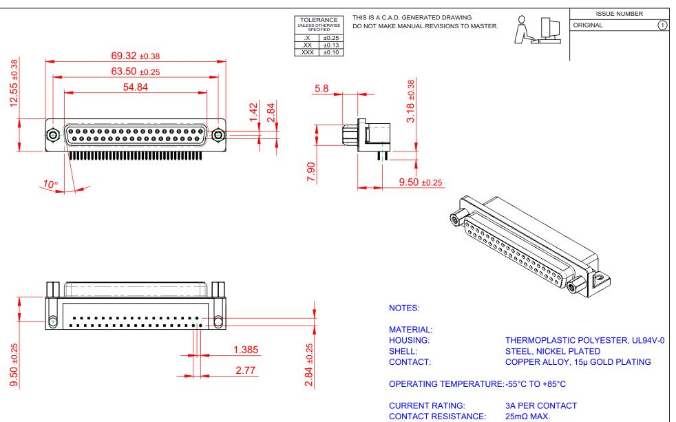
**INSULATOR RESISTANCE:** 5000MΩ min. DIELECTRIC WITHSTANDING VOLTAGE: 1000V AC rms
