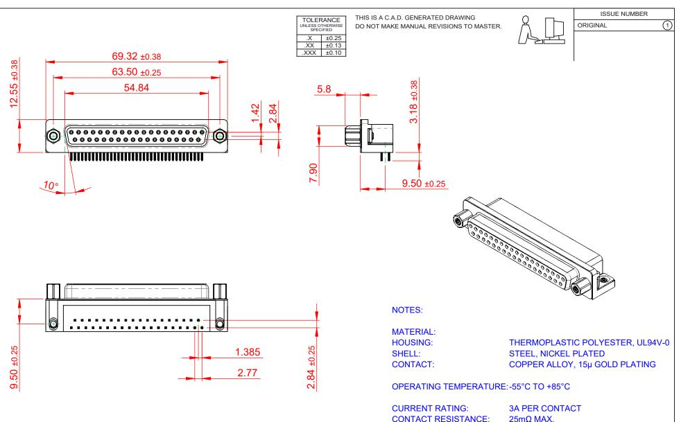
CONTACT RESISTANCE: 25mΩ MAX. **INSULATOR RESISTANCE:** 5000MΩ min. DIELECTRIC WITHSTANDING VOLTAGE: 1000V AC rms
