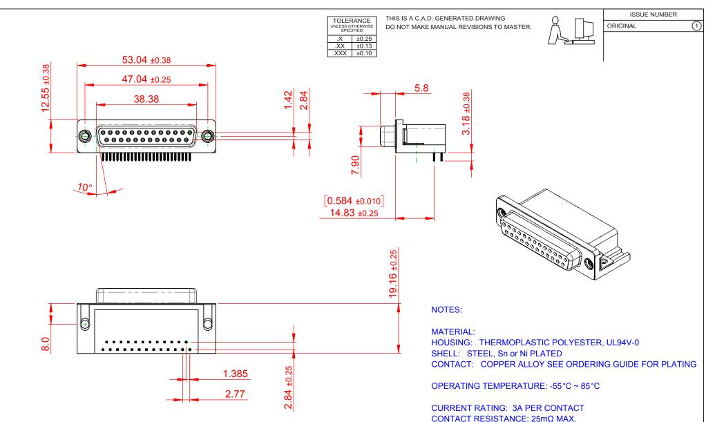
INSULATOR RESISTANCE:  $5000M\Omega$  min. **DIELECTRIC** WITHSTANDING VOLTAGE: 1000V AC rms
