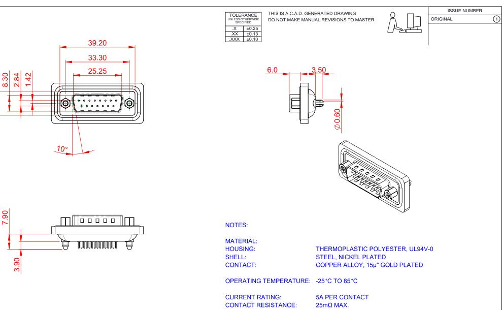
**INSULATOR RESISTANCE:** 5000MΩ min. DIELECTRIC WITHSTANDING VOLTAGE: 1000V AC rms
