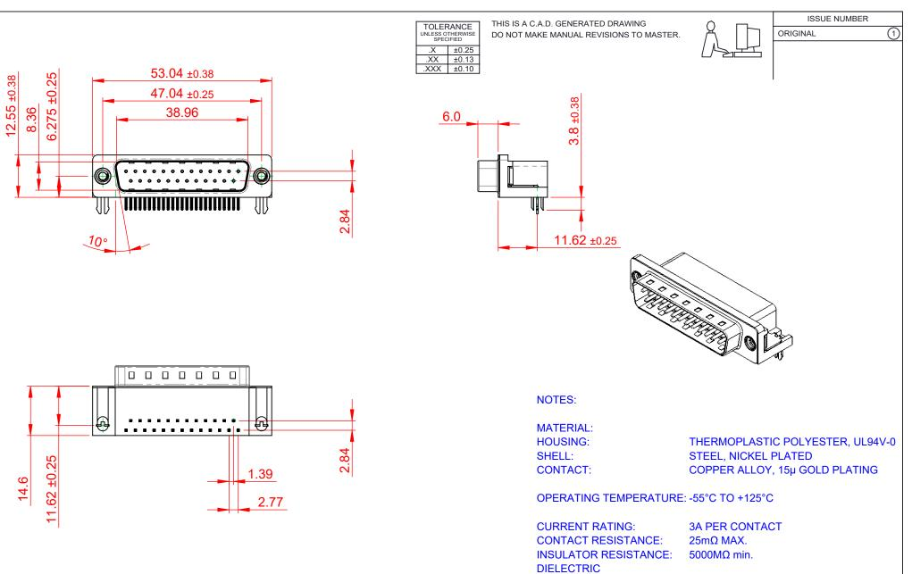
WITHSTANDING VOLTAGE: 1000V AC rms
