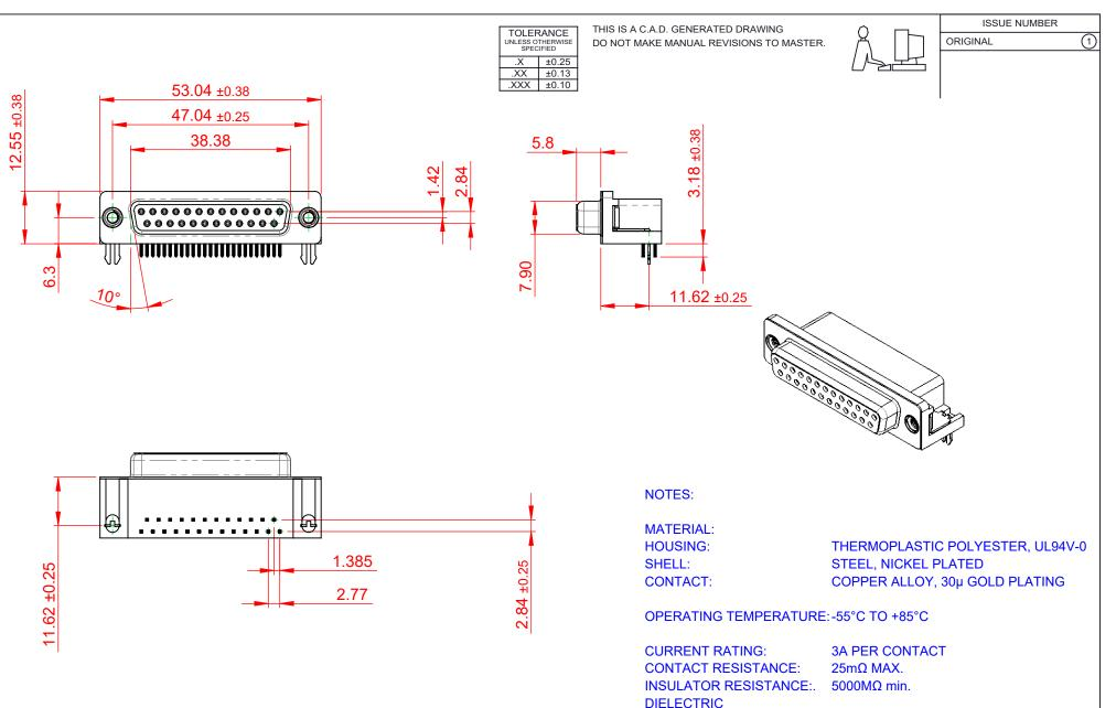
WITHSTANDING VOLTAGE: 1000V AC rms
