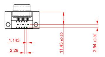
MATERIAL: HOUSING: PA6T, UL94V-0 SHELL: STEEL, Sn or Ni PLATED CONTACT: PRECISION MACHINED COPPER ALLOY SEE ORDERING GUIDE FOR CONTACT PLATING
