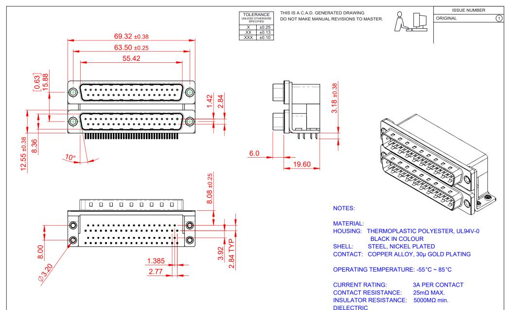
WITHSTANDING VOLTAGE: 1000V AC rms
