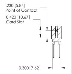
ACAD REFERENCE NO. 725-ENG MASTER 725 Series Ultra-Mate Card Edge Connector - Press Fit SEGAHOM:3A:9A DRAWN: J.LEE Part Number: 725-014-540-201 CHECKED: DATE: **EDAC INC** SCALE: SHEET 1 OF 1 THESE DRAWINGS AND SPECIFICATIONS ARE THE PROPERTY OF EDAC INC.,AND TORONTO, ONTARIO SHALL NOT BE REPRODUCED, OR COPIED DRAWING NUMBER **ISSUE** CANADA OR USED AS THE BASIS FOR THE 725-ENG MASTER MANUFACTURE OR SALE OF APPARATUS YOUR CONNECTION TO QUALITY & SERVICE WITHOUT WRITTEN PERMISSION.
