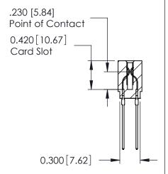
725 Series Ultra-Mate Card Edge Connector - Press Fit ACAD REFERENCE NO.
