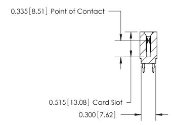
ACAD REFERENCE NO. 745 Series Ultra-Mate Card Edge Connector - Press Fit DRAWN: J.LEE Part Number: 745-050-525-201 CHECKED: **EDAC INC** SCALE: THESE DRAWINGS AND SPECIFICATIONS ARE THE PROPERTY OF EDAC INC.,AND TORONTO, ONTARIO SHALL NOT BE REPRODUCED, OR COPIED DRAWING NUMBER CANADA OR USED AS THE BASIS FOR THE 745-ENG MASTER MANUFACTURE OR SALE OF APPARATUS YOUR CONNECTION TO QUALITY & SERVICE WITHOUT WRITTEN PERMISSION.
