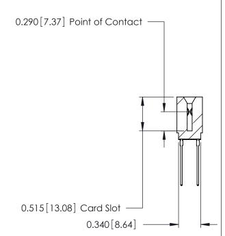
ACAD REFERENCE NO. 746 Series Ultra-Mate Card Edge Connector - Press Fit DRAWN: J.LEE DATE: AUG 20/09 Part Number: 746-038-553-201 CHECKED: DATE: **EDAC INC** SCALE: SHEET 1 OF 1 THESE DRAWINGS AND SPECIFICATIONS ARE THE PROPERTY OF EDAC INC., AND TORONTO, ONTARIO SHALL NOT BE REPRODUCED, OR COPIED DRAWING NUMBER CANADA OR USED AS THE BASIS FOR THE 746-ENG MASTER MANUFACTURE OR SALE OF APPARATUS YOUR CONNECTION TO QUALITY & SERVICE WITHOUT WRITTEN PERMISSION.
