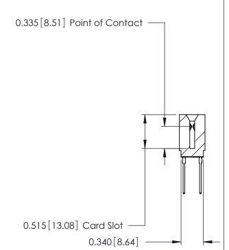
ACAD REFERENCE NO. 746-ENG MASTER 746 Series Ultra-Mate Card Edge Connector - Press Fit DRAWN: J.LEE DATE: AUG 20/09 Part Number: 746-044-545-201 CHECKED: DATE: **EDAC INC** SCALE: SHEET 1 OF 1 THESE DRAWINGS AND SPECIFICATIONS ARE THE PROPERTY OF EDAC INC.,AND TORONTO, ONTARIO SHALL NOT BE REPRODUCED, OR COPIED DRAWING NUMBER CANADA OR USED AS THE BASIS FOR THE 746-ENG MASTER MANUFACTURE OR SALE OF APPARATUS YOUR CONNECTION TO QUALITY & SERVICE WITHOUT WRITTEN PERMISSION.
