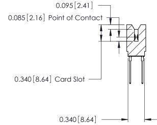
ACAD REFERENCE NO. 746-ENG MASTER 746 Series Ultra-Mate Card Edge Connector - Press Fit DRAWN: J.LEE DATE: AUG 20/09 Part Number: 746-046-540-606 CHECKED: DATE: **EDAC INC** SCALE: SHEET 1 OF 1 THESE DRAWINGS AND SPECIFICATIONS ARE THE PROPERTY OF EDAC INC.,AND TORONTO, ONTARIO SHALL NOT BE REPRODUCED, OR COPIED DRAWING NUMBER CANADA OR USED AS THE BASIS FOR THE 746-ENG MASTER MANUFACTURE OR SALE OF APPARATUS YOUR CONNECTION TO QUALITY & SERVICE WITHOUT WRITTEN PERMISSION.
