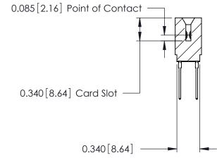
ACAD REFERENCE NO. 746 Series Ultra-Mate Card Edge Connector - Press Fit DRAWN: Part Number: 746-066-540-601 **EDAC INC** THESE DRAWINGS AND SPECIFICATIONS ARE THE PROPERTY OF EDAC INC.,AND TORONTO, ONTARIO SHALL NOT BE REPRODUCED, OR COPIED CANADA OR USED AS THE BASIS FOR THE MANUFACTURE OR SALE OF APPARATUS YOUR CONNECTION TO QUALITY & SERVICE
