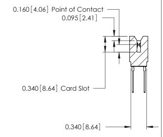
ACAD REFERENCE NO. 746 Series Ultra-Mate Card Edge Connector - Press Fit DRAWN: Part Number: 746-068-545-606 CHECKED: **EDAC INC** THESE DRAWINGS AND SPECIFICATIONS ARE THE PROPERTY OF EDAC INC.,AND TORONTO, ONTARIO SHALL NOT BE REPRODUCED, OR COPIED CANADA OR USED AS THE BASIS FOR THE MANUFACTURE OR SALE OF APPARATUS
