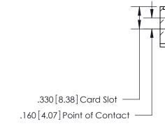
Card Slot Accepts .054 [1.37] to .070 [1.78] Thick P.C. Board
